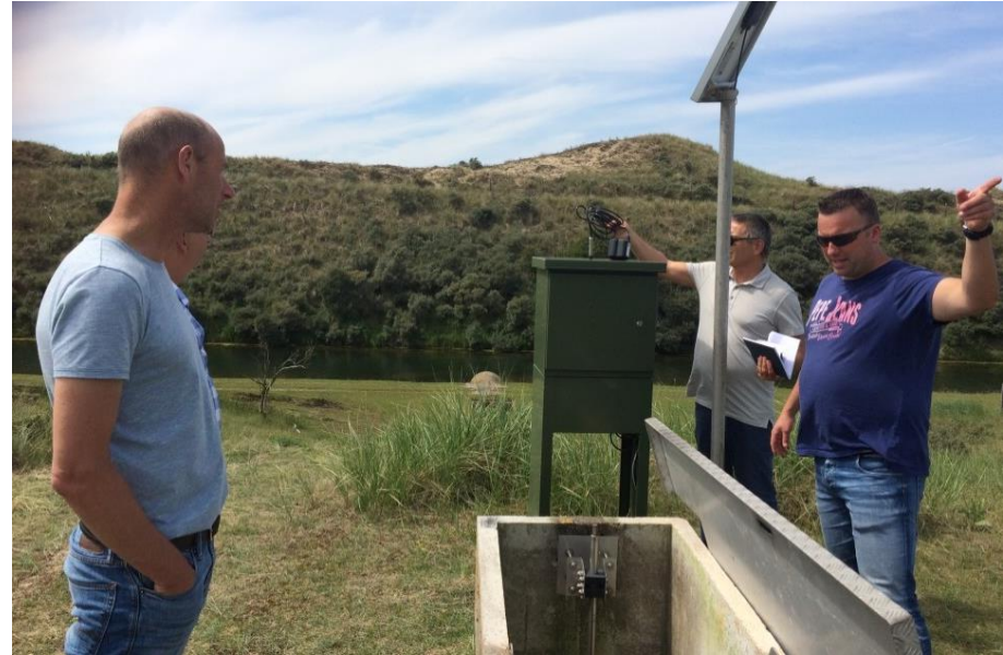
Testing surface water and groundwater readings via LPWAN in the Amsterdamse Waterleidingduinen.
