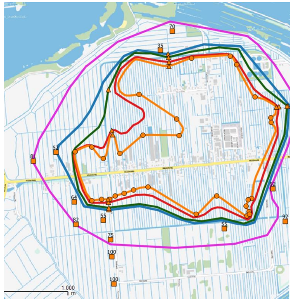
The boundary between salt water and fresh water at various depths in the Horstermeerpolder. At the centre of the polder, the boundary is closer to ground level than in the outer sections
